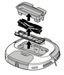
1. Press brush roll release button on top of robot and lift center unit out.
